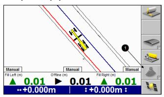
6. If the system has a single sonic tracer installed, press softkey **1** to enable 3D plus sonic tracer mode.
