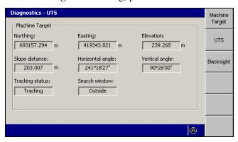
The first Diagnostics - UTS screen is Machine Target. This is the screen that appears if you press Machine Target. The fields in this screen are described below:
