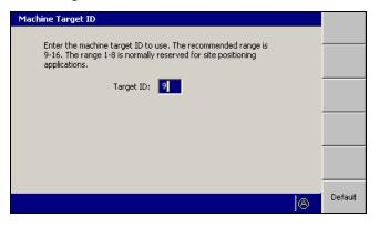
Note - The Target ID softkey is only available when the UTS is stopped.
