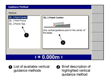
Figure 3.2 Example of a 3D Guidance Method dialog
