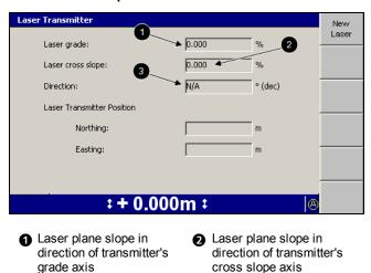
Figure 5.2 Example Laser Transmitter dialog
