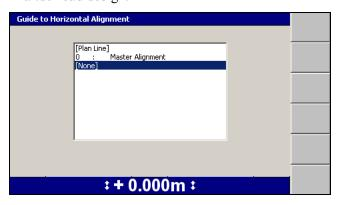
4. Highlight the required alignment option. The following options may be available in the Guide to Horizontal Alignment dialog, depending on the type of design loaded:
