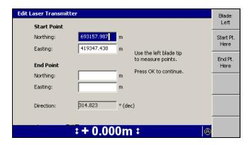
This dialog lets you specify the direction of the "grade" axis by defining a line segment that runs parallel to, and in the same direction as, the "grade" axis.
