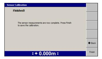
10. To accept the calibration and return to the *Calibrate Sensors* menu, press Finish. If you want to redo all or part of the calibration, press the back arrow softkey to return to the previous screen. To escape to the Calibrate Sensors menu without saving the calibration, press 2.
