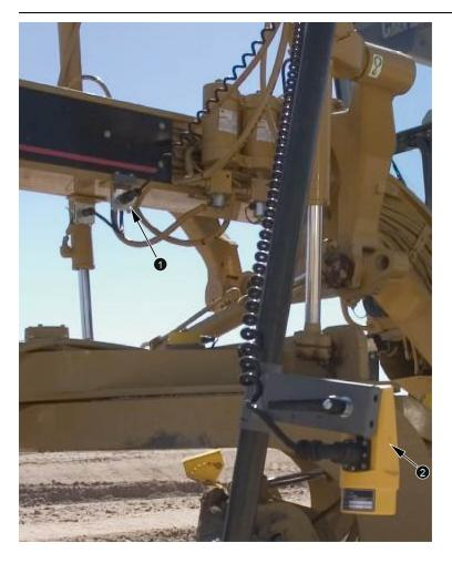
System harness nose connector on gooseneck Sonic tracer
