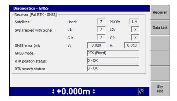
The first Diagnostics – GNSS screen is the Receiver screen, if you have a single-GNSS receiver system. The following table describes the fields in this screen.
