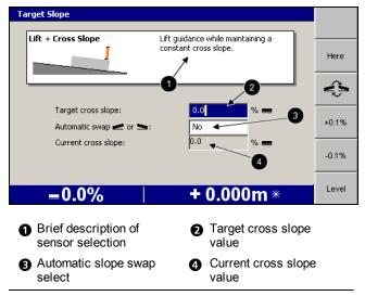
Figure 4.7 Example cross slope setup dialog
