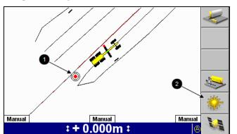
The plan view guidance shows the location of the laser transmitter (1):
