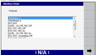
2. Use the arrow keys to select the wireless mode from the list of available protocols, then press or \_\_\_\_\_. The *Wireless mode - Baud Rate* screen appears:
