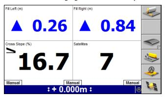
**Note** – Up to 10 text view items can be displayed in full screen view and the text size scales automatically to fit the available screen space.
