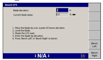
4. Enter the elevation of the benchmark into the *Blade elevation* field.
