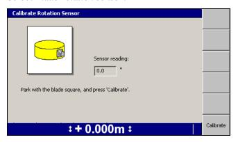
2. Make sure that the machine is parked on flat ground and that the blade is square.
