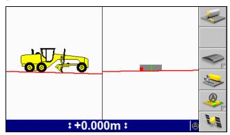
**Note** – Split view replaces both the cross-section and profile views. When split view is available, you cannot view the cross-section and profile views as full screen views.
