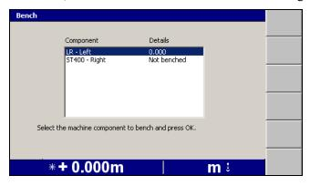
Note – The contents of the Bench menu will vary depending on the number of laser receivers and sonic tracers being used by the system.
