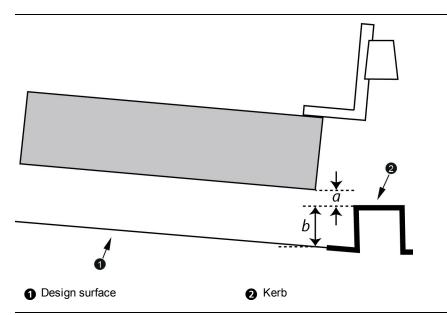
Figure 4.3 Measurements for benching a sonic tracer over a kerb
