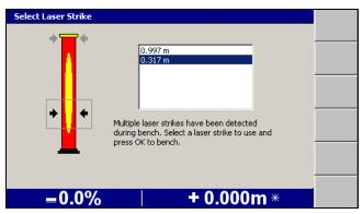
Note – By default, laser strikes must be at least 100 mm (4 inches) apart to be distinguished as coming from separate laser transmitters. It may take a few seconds for the system to gather enough data to distinguish between clusters of laser strikes from different transmitters. For this reason, there may be a short delay between pressing the Bench Left or Bench Right softkey, and the appearance of the Select Laser Strike dialog.
