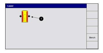
Laser strike indication in the Laser dialog for Figure 4.4 a manual mast
