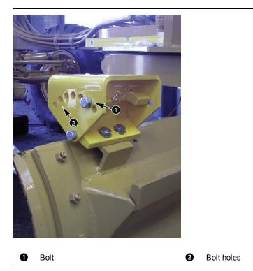
Figure 3.1 Motor grader rotating mast mount
