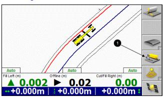
1. From any guidance screen press the **Offsets** softkey (**①**). The *Vertical Offset* dialog appears:
