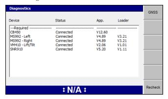
Devices showing as **Not Required** are connected, but are not required by the currently configured system.
