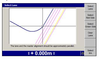
The selected line is shaded double-thick blue and the lane guidance softkeys are displayed.
