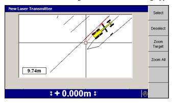
Use the arrow keys to move the cross-hairs around the screen. As the cross-hairs move, the distance from the focus point on the cutting edge to the position indicated by the cross-hairs appears.
