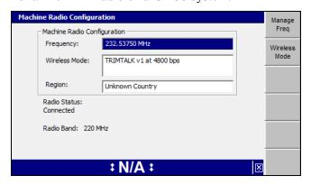
Use the arrow keys to select the Network or Frequency setting required. To save the changes, press (\*\*); to exit without saving changes, press (\*\*).
