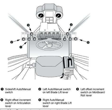
Figure 2.6 Typical motor grader remote switch locations
