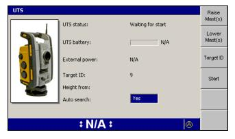
2. Press Raise Mast(s) and/or Lower Mast(s) to position the mast so that line of sight with the UTS target is maintained, while at the same time keeping the mast low enough to minimize mast vibration. The maximum operating
