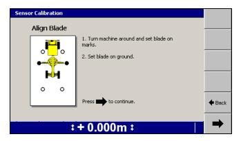
5. Raise the blade and then turn the machine 180°. Do not articulate the machine or not lean the wheels and do not change the circle position while executing the turn.
