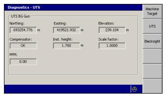
This screen displays the name of the point at which the UTS instrument was set up, if the point has a name, in the form UTS < name >. For example, UTS South. The fields within this screen are described below.
