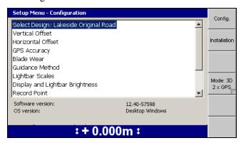
2. If required, press **Mode: <value>** to switch to a different mode. When a new sensor or device is added to or removed from the machine, the system automatically updates the mode values.
