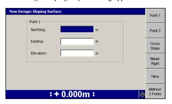
By default, the dialog shows the softkeys and fields needed to define a sloping surface using the 2-Points method.
