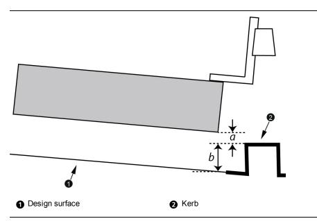
Figure 6.1 Measurements for benching a sonic tracer over a kerb
