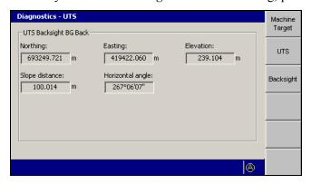
This screen displays information about the backsight taken to establish the orientation of the UTS instrument. The fields within this screen are described below.
