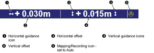
Figure 2.3 Example guidance setting area for a 3D system
