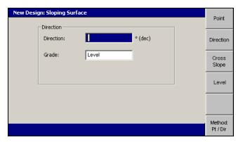
6. Edit the *Direction* field to specify the direction of the master alignment relative to Point 1.
