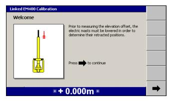
2. Press - The masts are driven to the bottom of their travel range. Once calibration has finished, the *Elevation* screen of the *Linked EM400 Calibration*
