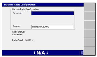
Note - This release of the system requires the use of SiteVision Office 7.4 or later for wireless communications over 900 MHz radios. For more information, refer to the GCS900 Grade Control System Site Supervisor's Manual.
