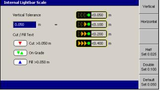
3. Press either **Vertical** or **Horizontal** to view the current vertical or horizontal tolerance settings respectively.
