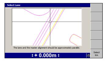
*Note* – When there is no master alignment in the current design, only the **Select** MA softkey is displayed.
