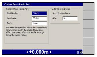
The control box's radio port is the communications port on the control box that connects to the communications port on the data radio. For the system to work, the settings in the *Control Box's Radio Port* dialog must match the communication port settings in the data radio. If these settings do not match, do the following:
