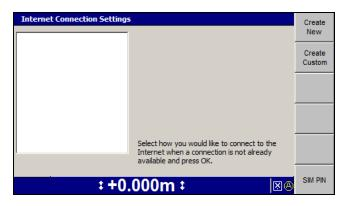
3. Press the up or down arrow keys on the control box to select how you would like to connect to the Internet and press [6].
