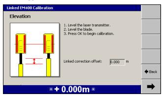
Level the laser transmitter and the blade.
