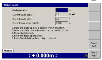
**Note** – Alternatively, to access the Bench Laser dialog press in and then from the Setup Menu – Configuration menu, select Bench.
