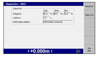
Note - The screen shown above is an example of a GNSS data link diagnostics screen for a single-GNSS system. The Data Link screen for dual-GNSS systems, or systems using a base station configured to send corrections in RTCM V3.0 format, will differ from that shown.
